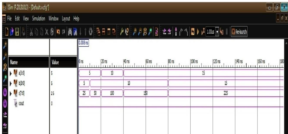
Figure 10:- Simulation result of 4x4 multiplier in decimal
