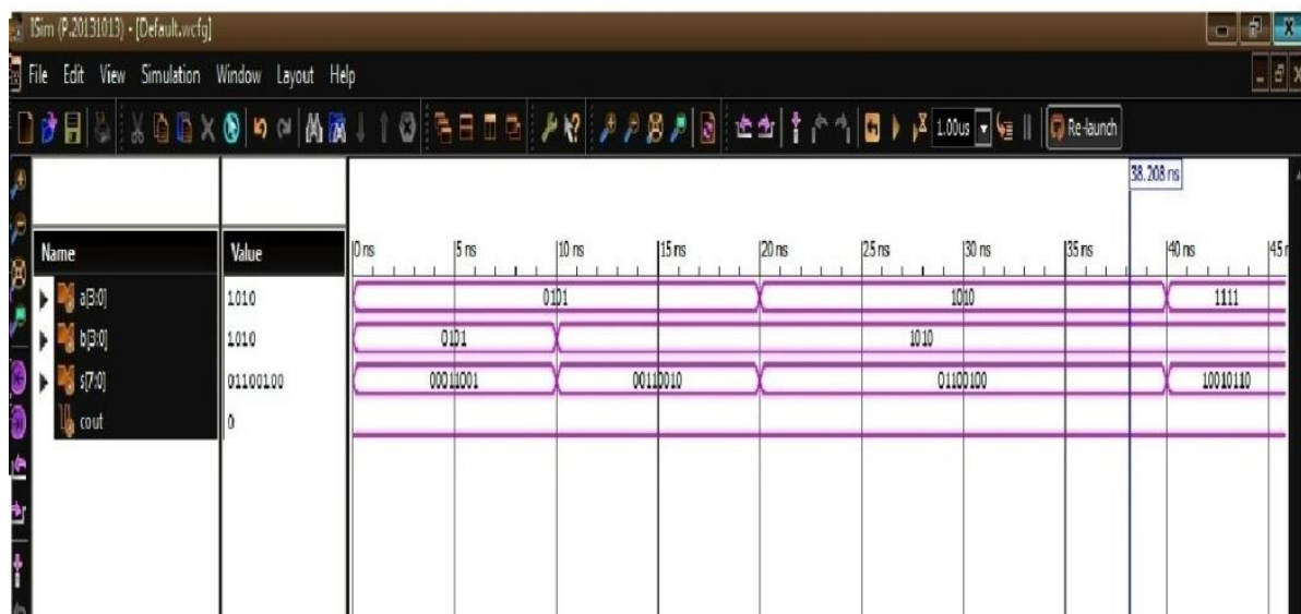
Figure 9:- Simulation result of 4x4 multiplier in binary
